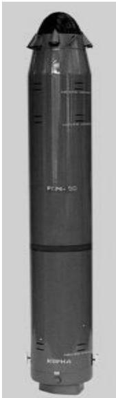
Designed to destroy strategic targets at intercontinental ranges. Adopted for operation by the Navy in 1977. The missile was installed aboard the 667BDR nuclear submarines (16 missiles per submarine).
