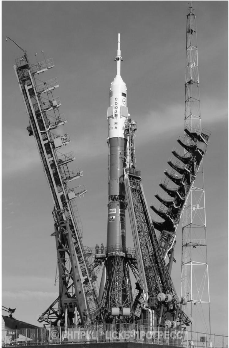
where cosmonauts operated for launch and reentry of the Soyuz space craft. This module would separate on reentry from the others and would have its own heat resistant coating. The orbital module was the habitation module for early missions and is still used for that purpose as well as a space for performing experiments. The last module is the propulsion and instrumentation module. This module holds not only the propulsion drive but also holds the instrumentation needed for the mission.
