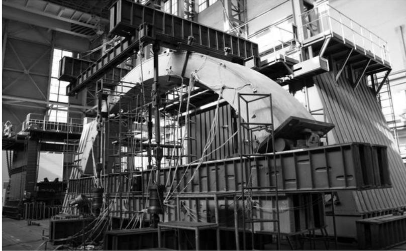
The complex is dedicated for static and cyclic tests. The tests are conducted on strength test stands, reinforced floor and wall.
